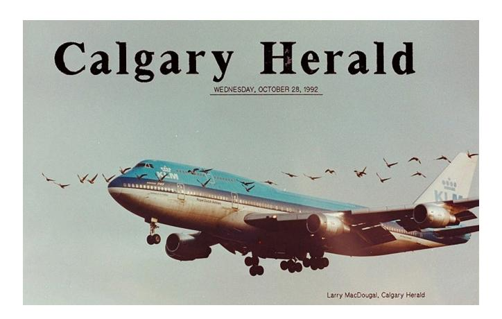
Figure 3 Boeing 747 Encounter with a Flock of Canada Geese just prior to Bird Ingestion in Outboard Left Wing Engine. Birds appear to be unaware of aircraft's presence.
