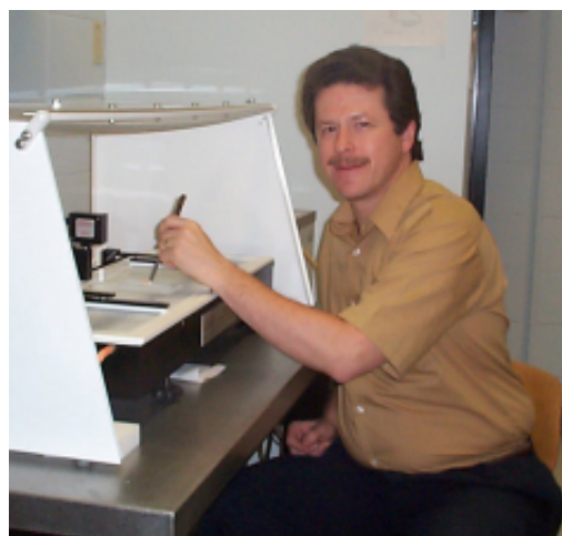
Dr. Ducharme is making two-dimensional ferroelectric films with the Langmuir-Blodgett.
