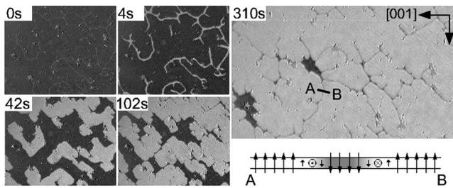
FIG. 6. Evolution of the magnetization of 3 ML Fe/Cu(001) after a magnetic field of  $H = -0.97$  mT was applied at  $t = 0$  s. After 310 s narrow lines of original magnetization remain due to the formation of 360 deg walls preventing the fully saturated opposite magnetization state. Image size:  $400 \times 300 \mu\text{m}^2$ .
