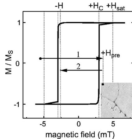
FIG. 2. MOKE magnetization loop of 3 ML Fe/Cu(001) at 120 K. The fields relevant for the after-effect measurements are indicated. Inset: Kerr image taken at  $H_{pre}$  showing nucleated domains. (Image size  $70 \times 70 \mu\text{m}^2$ .)
