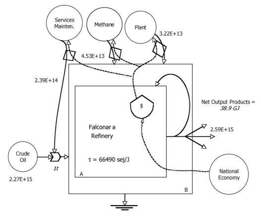
Fig. 1 – An energy diagram of the Falconara refinery system (emergies of the inputs – in sej – are in bold). The analysis was performed using boundary B. Tau,  $\tau$ , represents the transformity of the generic oil derivative.
