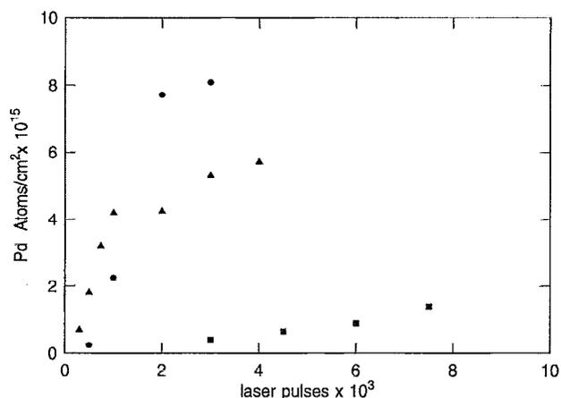
FIG. 3. Pd deposition vs number of pulses as measured by RBS. 248 nm light, 300 mJ/cm<sup>2</sup> (triangles) and 210 mJ/cm<sup>2</sup> (dots); 308 nm light, 300 mJ/cm<sup>2</sup> (squares).
