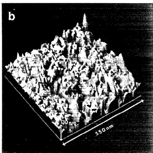
FIG. 1. AFM scans on seeded samples (a) after 3000 pulses at 300 mJ/cm<sup>2</sup> with the 308 nm line; (b) after 2000 pulses at 210 mJ/cm<sup>2</sup> with the 248 nm line. The scanned area was 550×550 nm.
