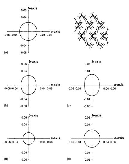
FIG. 4. Linear compressibility diagrams for RDX in the *ab* crystallographic plane for (a) this work, (b) Schwarz *et al.*, (c) Haussühl, (d) Ye *et al.*, and (e) Sewell and Bennett. The projection of RDX molecules in the unit cell for this plane is shown in the upper-right corner. Units are in GPa<sup>-1</sup>.
