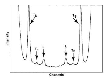
FIG. 1. Example Brillouin spectrum of RDX for the (0.707 10, 0.707 10, 0.000 00) phonon. The transverse slow  $(T_s)$ , transverse fast  $(T_f)$ , and longitudinal modes (L) are labeled. The free spectral range is 1.369 cm<sup>-1</sup>. Polarization is laboratory Vertical-Vertical.
