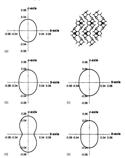
FIG. 6. Linear compressibility diagrams for RDX in the *bc* crystallographic plane for (a) this work, (b) Schwarz *et al.*, (c) Haussühl, (d) Ye *et al.*, and (e) Sewell and Bennett. The projection of RDX molecules in the unit cell for this plane is shown in the upper-right corner. Units are in GPa<sup>-1</sup>.
