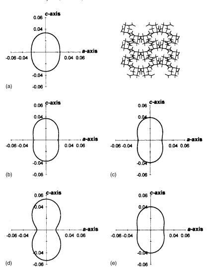
FIG. 5. Linear compressibility diagrams for RDX in the *ac* crystallographic plane for (a) this work, (b) Schwarz *et al.*, (c) Haussühl, (d) Ye *et al.*, and (e) Sewell and Bennett. The projection of RDX molecules in the unit cell for this plane is shown in the upper-right corner. Units are in GPa<sup>-1</sup>.
