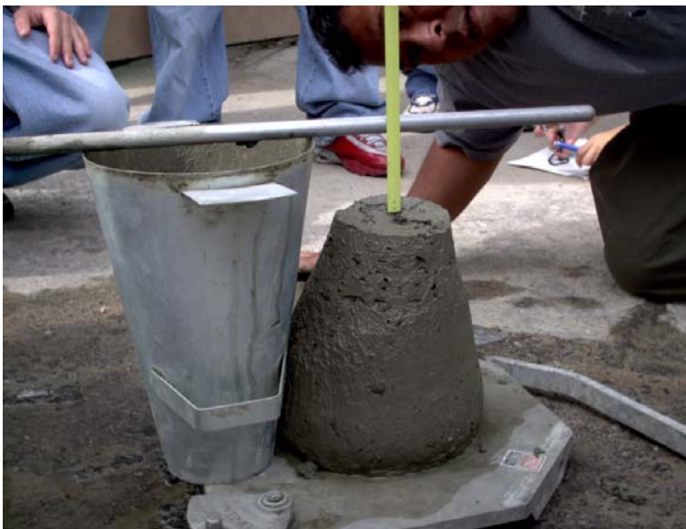
Fig. 2.3 Fresh Concrete Slump Test
