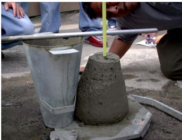
Fig. 2.3 Fresh Concrete Slump Test
