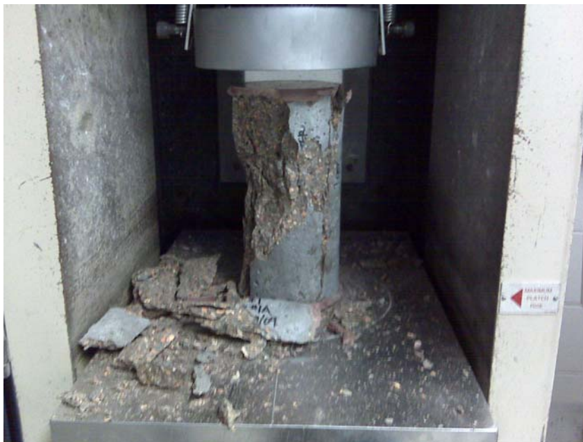
Fig. 2.5 Completed Compression Test
