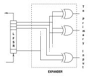
Fig. 2. Schematic of expander
