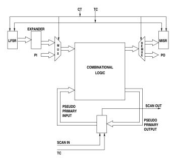
Fig. 1. Proposed test architecture
