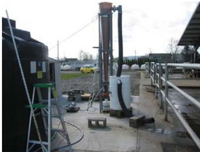
Business Innovation Research (SBIR) program and Washington Technology Center, used a fluidized bed to crystallize phosphorus from lagoon water into struvite (P + magnesium). The granular struvite can be marketed for use in inorganic fertilizers. The second output, reduced P lagoon water, can be utilized in the farm's cropping system.
