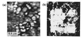
FIG. 5. Simultaneously obtained (a) topographic and (b) piezoresponse images of the fatigued PZT/Pt heterostructure. The bright square of  $1\times1~\mu\text{m}^2$ , produced by moving the SFM tip while applying a negative 15 V dc voltage, represents a negatively polarized region. Unswitchable crystallites appear as dark areas inside the white square region.
