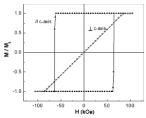
Fig. 4. Hysteresis loops of core-shell structure.
