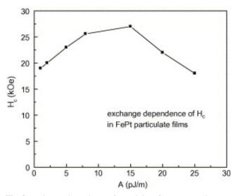
Fig. 8. Exchange-dependence of coercivity of nanocomposites.
