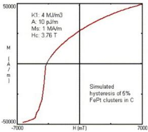
Fig. 5. Simulated hysteresis for assembly of isolated nanoclusters.
