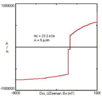
Fig. 7. Simulated hysteresis for the FePt matrix system.
