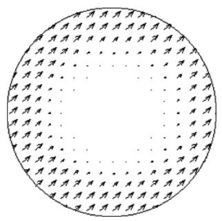
**Fig. 1.** Real-space spin structure of a core–shell particle  $(R_{core} = R - \Delta R)$ .
