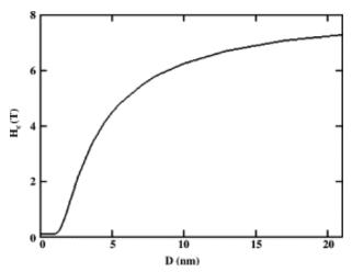
**Fig. 3.** Coercivity as a function of the particle diameter D = 2R for typical L1<sub>0</sub> parameters.
