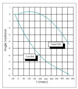
Fig. 5. Rotation angles of colliding billiard balls simulated by *Interactive Physics*. Initial velocity of cue ball = 1 m/s. Frictional coefficients = 0.08. See Fig. 4.
