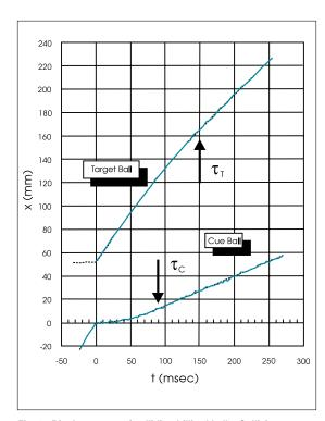
Fig. 2. Displacements of colliding billiard balls. Collision occurs at t= 0. Raw data and least-squares fitted curves are shown. Skidding of cue ball stops at time  $\tau_{\rm c}$ ; skidding of target ball stops at  $\tau_{\rm T}$ .
