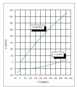
Fig. 4. Displacements of colliding billiard balls simulated by *Interactive Physics*. Initial velocity of cue ball = 1 m/s. Frictional coefficients = 0.08.
