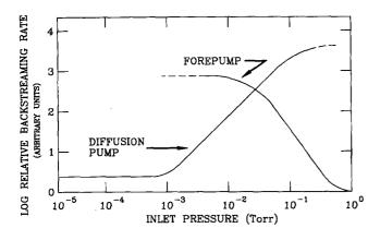
Fig. 4. Mechanical forepump and diffusion pump backstreaming rates vs their respective inlet pressures (see the text). After Fig. 10.2, Ref. 5; see also Ref. 16.
