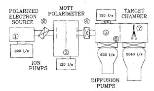
Fig. 1. Schematic view of vacuum system showing elements relevant to the text: (1) RGA in source; (2) manual bakeable in-line copper-sealed valve; (3) collimators and baffles which aid in differential pumping of the Mott polarimeter; (4) electropneumatic viton-sealed gate valve; (5) target RGA; (6) target-gas containment baffle; (7) effusive gas target. A 120  $\ell$ /s ion pump on top of the target chamber is used to maintain vacuum when the diffusion pump butterfly valves are closed.
