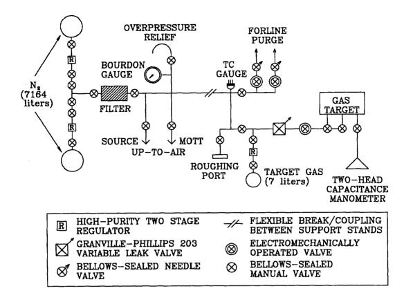
Fig. 3. Target/purge gas handling system.
