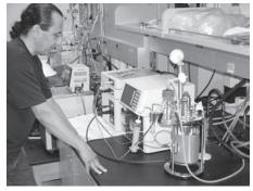
Chemical Engineer Hossein Noureddini studies adding the enzyme phytase during ethanol production, which would remove phosphorus from the organic compounds. This is just one way UNL researchers are working to reduce phosphorus in manure and in distillers grain and corn gluten feed.
