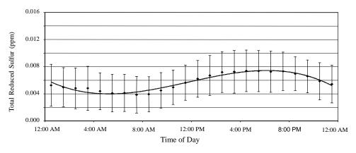
Figure 4. Average TRS concentration (reported as an H<sub>2</sub>S equivalent) vs. time of day for feedlot no. 3 during spring 2001.
