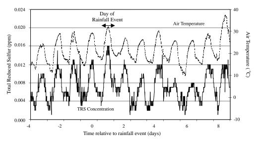
Figure 5. Impact of rainfall on TRS concentration (reported as an H<sub>2</sub>S equivalent) for feedlot no. 3 (Event 5, 10-21 August).
