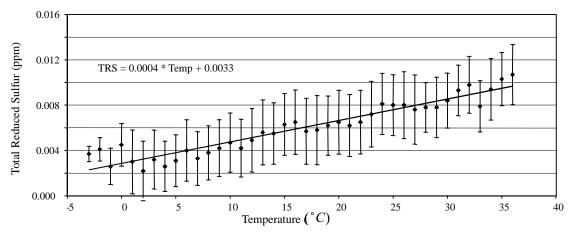
Figure 2. Average TRS concentration ( $\pm$  1 standard deviation) vs. air temperature for feedlot no. 3 during spring 2001. TRS is reported as  $H_2S$  equivalent.
