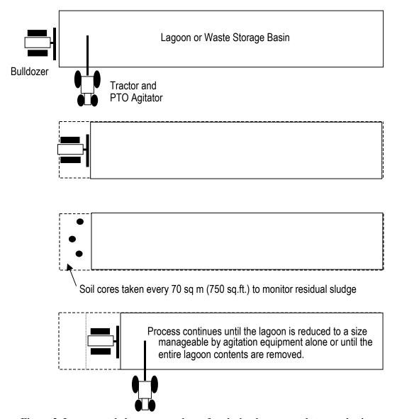
Figure 2. Incremental closure procedures for closing lagoons and storage basins.
