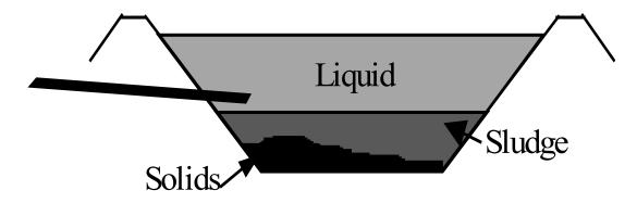
Figure 3. Cross-section of an anaerobic lagoon.
