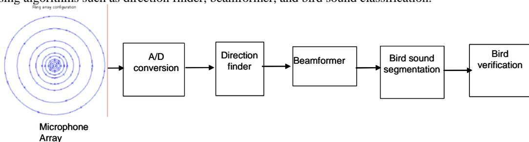
Figure 1 Proposed automated bird monitoring and recognition system.
