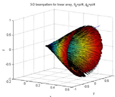
Figure 12 Three-D beampattern of compound linear array.
