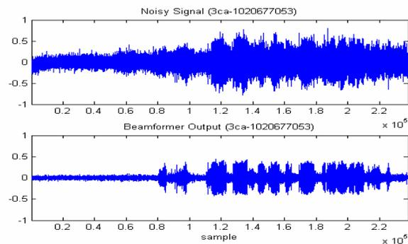
Figure 21 Signals before beamforming and after beamforming.
