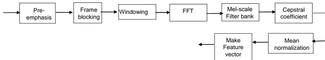
Figure 14 Preprocessing steps in the feature extraction subsystem.
