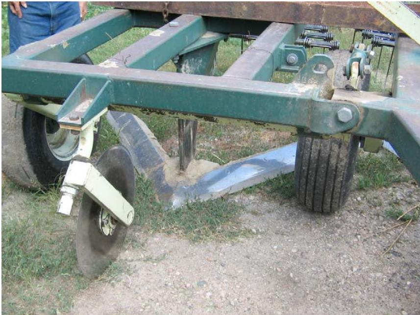
Photograph 4. The blade plow gets under the top layer of residue, but leaves it on top of the soil. This farmer uses the blade plow to control weeds and provide a better cover in his fallow rotation to conserve moisture. (Melissa Melvin and Jeff Nothwehr, NDMC, 2005)
