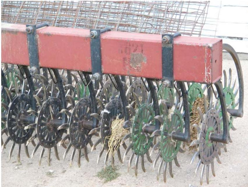
Photograph 3. The above picture show a rotary hoe. This rotary hoe is used by an organic farmer to minimize soil disturbance and control weeds in his fields without the use of pesticides. (Melissa Melvin and Jeff Nothwehr, NDMC, 2005)
