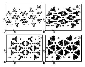
FIG. 4. Projections of the atomic positions along the b axis in the average structure of  $\text{Ca}_2\text{SiO}_4$  obtained from heating up the phase  $\gamma$ . (a) Phase  $\gamma$  at 1000 K, (b) phase  $\gamma$  at 1390 K, (c) phase  $\alpha'_H$  at 1600 K, (d) phase  $\alpha$  at 1870 K.
