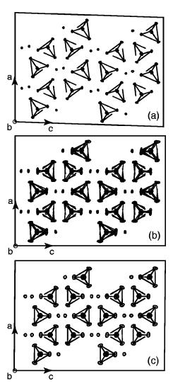
FIG. 6. Projections of the atomic positions along the b axis in the average structure of  $\text{Ca}_2\text{SiO}_4$  obtained from heating up the phase  $\beta$ . (a) Phase  $\beta$  at 850 K, (b) phase  $\alpha_I'$  at 1050 K, (c) phase  $\alpha_H'$  at 1630 K.
