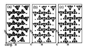
FIG. 7. Projections of the atomic positions along the c axis in the average structure of  $Ca_2SiO_4$  obtained from heating up the phase  $\beta$ . (a) Phase  $\beta$  at 850 K, (b) phase  $\alpha'_L$  at 1050 K, (c) phase  $\alpha'_H$  at 1630 K.
