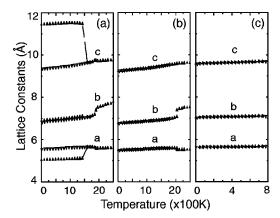
FIG. 2. Lattice constants of the unit cell as a function of temperature for the MD run. (a)  $Ca_2SiO_4$ , starting from phase  $\gamma$ , (b)  $Ca_2SiO_4$ , starting from phase  $\beta$ ; (c)  $Sr_2SiO_4$ . Solid up triangles: heating up; hollow down triangles: cooling down.
