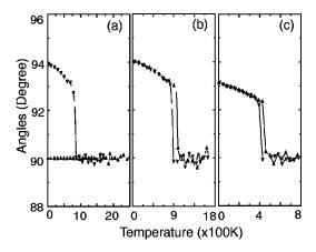
FIG. 3. Angle between lattice vectors a and c as a function of temperature for the MD run. (a) Ca<sub>2</sub>SiO<sub>4</sub>, starting from phase  $\gamma$ ; (b) Ca<sub>2</sub>SiO<sub>4</sub>, starting from phase  $\beta$ ; (c) Sr<sub>2</sub>SiO<sub>4</sub>. Solid up triangles: heating up; hollow down triangles: cooling down.
