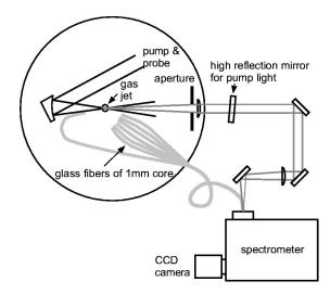
FIG. 1. Setup of angle-resolved spectroscopy for detecting the spectra of Raman scattering or collective Thomson scattering. The fiber array was removed from the entrance slit of the spectrometer when the direct forward channel (using lenses) was used. The spectrometer was a prism spectrometer when a low spectral resolution and a large range were needed, and was a 1200 lines/mm grating spectrometer when a high spectral resolution was needed
