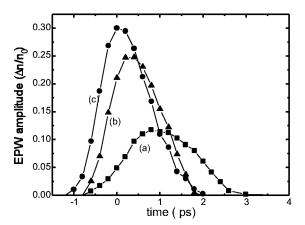
FIG. 9. Spatially averaged temporal evolution of the EPW amplitude for various laser powers at a plasma density of  $3.7 \times 10^{19} \, \mathrm{cm}^{-3}$ : (a) 1 TW, (b) 1.9 TW, and (c) 3.2 TW. The number of electrons accelerated in each case is  $10^7$ ,  $10^8$ , and  $10^9$ , respectively.
