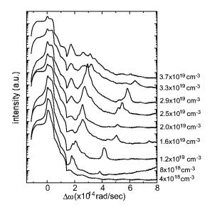
FIG. 2. Spectra of Raman forward scattering in the 15° direction for various plasma densities at a fixed laser power of 2.5 TW. Note that the intensity scale is logrithmic and that the curves are vertically displaced for ease of viewing.
