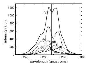
FIG. 12. Spectra of the scattered probe light at various angles for 3 TW laser power,  $3.7 \times 10^{19} \, \mathrm{cm^{-3}}$  plasma density and 20 ps probe delay: (a) 25°, (b) 35°, (c) 45°, (d) 55°, and (e) 65°. The vertical line indicates the unshifted probe central wavelength. Note that the bumps on the shoulder originate from the original probe spectrum which is monitored with the 165° channel, (f), which detected the probe light scattered from the nozzle.
