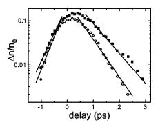
FIG. 8. Amplitude of the plasma wave as a function of probe delay at 1.5 TW pump power and  $3.7 \times 10^{19} \, \mathrm{cm}^{-3}$  plasma density. Solid squares (open circles) represent the amplitudes derived from anti-Stokes (Stokes) satellites. The exponential fits of the growth and decay rates are also shown.
