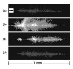
FIG. 11. Side images of the first Stokes–Thomson satellite at various probe delays for 2.5 TW laser power and  $3.7\times10^{19}\,\mathrm{cm}^{-3}$  plasma density: (a)  $-1\,\mathrm{ps}$ , (b)  $+0.2\,\mathrm{ps}$ , (c)  $+0.6\,\mathrm{ps}$ , and (d)  $+1.6\,\mathrm{ps}$ . The arrow indicates the direction of laser propagation.
