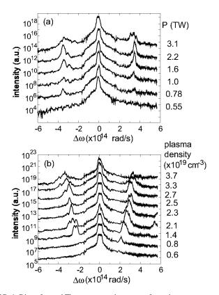
FIG. 6. Direct forward Thomson scattering spectra for various pump powers at  $3.7 \times 10^{19}$  cm<sup>-3</sup> plasma density, (a), and for various plasma densities at 3 TW pump power, (b). The probe delay is zero. Note that the intensity scale is logrithmic and that the curves are vertically displaced for ease of viewing.
