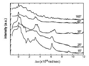
FIG. 4. Spectra of Raman forward scattering for various angles of observation at 2.5 TW laser power and  $3.7 \times 10^{19}$  cm<sup>-3</sup> plasma density. Note that the intensity scale is logrithmic and that the curves have been vertically displaced for ease of viewing.
