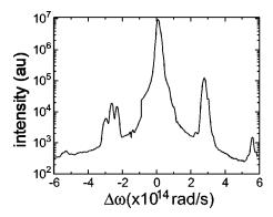
FIG. 5. Direct forward Thomson scattering spectrum for 3 TW pump power,  $2.3\times10^{19}\,\mathrm{cm^{-3}}$  plasma density, and zero probe delay.
