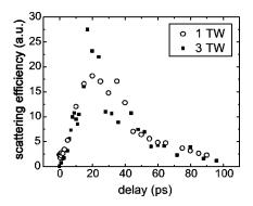
FIG. 14. Temporal evolution of the scattered intensity of the probe near the probe wavelength for various laser powers at  $25^{\circ}$  and a plasma density of  $3.7 \times 10^{19}$  cm<sup>-3</sup>.
