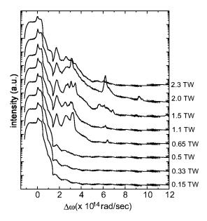
FIG. 3. Spectra of Raman forward scattering in the  $15^{\circ}$  direction for various laser powers at a fixed plasma density of  $3.7 \times 10^{19} \, \mathrm{cm}^{-3}$ . Note that the intensity scale is logrithmic and that the curves are vertically displaced for ease of viewing.
