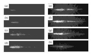
FIG. 15. Side imaging of the scattered intensity near the probe wavelength for various probe delays at 2.5 TW laser power and  $3.7 \times 10^{19}$  cm<sup>-3</sup> plasma density: (a) +0.3 ps, (b) +0.9 ps, (c) +1.9 ps, (d) +3.4 ps, (e) +10 ps, (f) +20 ps, (g) +40 ps, (h) +60 ps. The laser pulses propagate from left to right.
