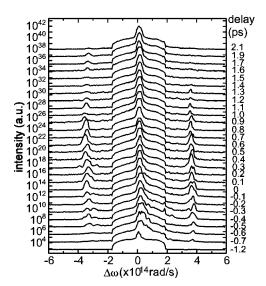
FIG. 7. Direct forward Thomson scattering spectra for various probe delays at 1.5 TW pump power and  $3.7\times10^{19}\,\mathrm{cm}^{-3}$  plasma density. Note that the intensity scale is logrithmic and that the curves are vertically displaced for ease of viewing.
