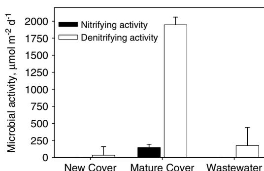
**Figure 1.** Rates of aerobic nitrifying and anaerobic denitrifying activity associated with lagoon geotextile cover samples and underlying wastewater from a swine lagoon ( $n = 3$ ). Comparisons were based upon a 0.5 cm thick layer. Source: DN Miller (unpublished).
