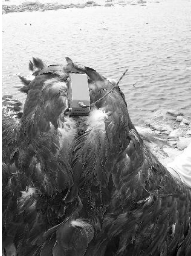
Figure 3: 95g PTT affixed in a pack-back fashion on a juvenile Bald Eagle.
