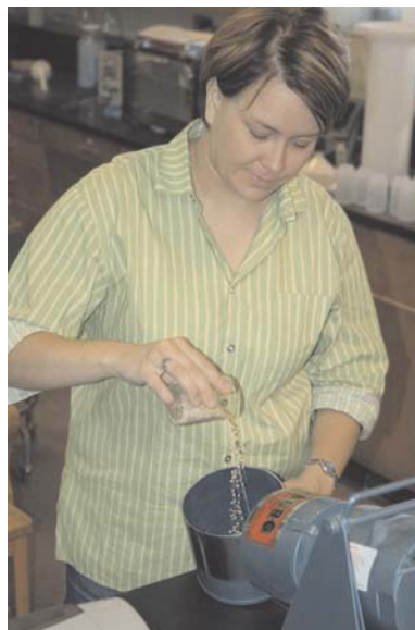
Laura pours grain sorghum into the bucket end of a seed scarifier.
