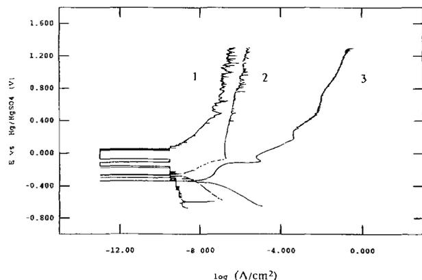
Fig. 5. Potentiodynamic curves measured on Ag paste treated with CH<sub>3</sub>-BTA/alcohol mixture measured after 4 months of storage in a closed container with a surplus of CH<sub>3</sub>-BTA powder (curve 1). Results on unprotected paste (curve 3) and on protected paste, measured hours after the treatment (curve 2) are given for a comparison.
