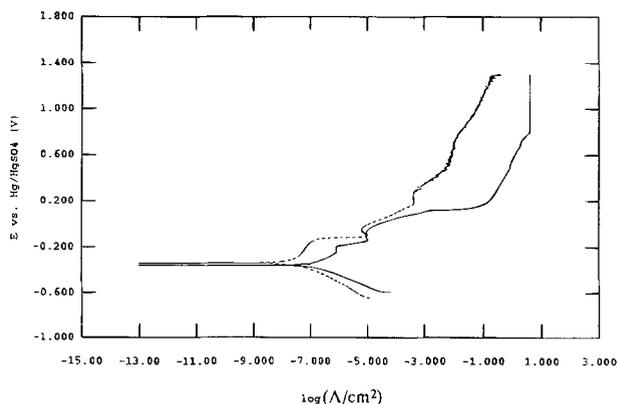
Fig. 1. Potentiodynamic polarization curves for an Ag foil (solid line) and Ag paste (dashed line) samples measured in a droplet of water.
