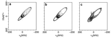
**Fig. 2.** <sup>79</sup>Br STREAQI spectra of l-tyrosine hydrobromide, simulated using the assumption (a) of a discrete jump between two static orientations and (b) continuous sample rotation; compared with (c) an experimental spectrum, obtained as described in the text.
