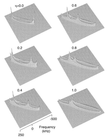
**Fig. 1.** Computed STREAQI spectra of a hypothetical substance with  $C_Q = 16$  MHz,  $v_0 = 150$  MHz, in the limit of slow-spinning at the magic angle, with a 2.4° jump during  $t_s$ .
