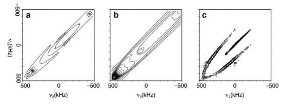
**Fig. 3.** <sup>79</sup>Br STREAQI spectra of l-leucine hydrobromide, simulated using the assumption of (a) a discrete jump between two static orientations and (b) continuous sample rotation; compared with (c) an experimental spectrum, obtained as described in the text.
