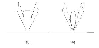
FIG. 4. Angular dependence of the steady-state intensity in the water as a function of angle for a normally incident longitudinal wave,  $x_T$ =0.5, without absorption: (a) total fluid intensity, (b) separation of longitudinal (solid line) and shear vertical (dashed line) contributions.
