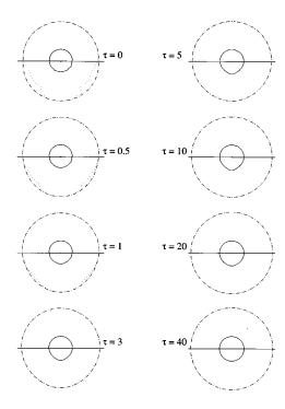
FIG. 5. Angular dependence of intensity as a function of dimensionless depth for iron in water,  $x_T$ =3.5, without absorption for the three modes  $I_L$  (solid line),  $I_{SV}$  (dotted), and  $I_{SH}$  (dot dash).
