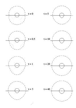
FIG. 6. Angular dependence of intensity as a function of dimensionless depth for aluminum in water,  $x_T$ =3.5, without absorption for the three modes  $I_L$  (solid line),  $I_{SV}$  (dotted), and  $I_{SH}$  (dot dash).
