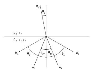
FIG. 2. Reflection and transmission of potential functions.
