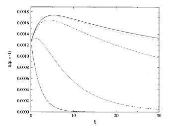
FIG. 7. Backscattered  $(\mu=-1)$  fluid intensity versus dimensionless time,  $\xi=c_T\kappa_T t$ , at dimensionless inner frequency  $x_T=0.5$  for different absorption rates: no absorption (solid line),  $\tilde{v}_T=0.001$  (dotted),  $\tilde{v}_T=0.01$  (dot dash), and  $\tilde{v}_T=0.111$  (small dash). The singly scattered solution without absorption is shown by the large dashes.
