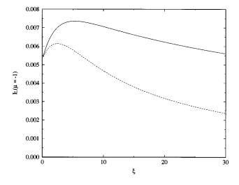
FIG. 8. Backscattered  $(\mu=-1)$  fluid intensity versus dimensionless time,  $\xi=c_T\kappa_T t$ , at dimensionless inner frequency  $x_T=0.5$  with (solid line) and without (small dash) the boundary. The solution with the boundary has been divided by the two transmission coefficients,  $T_{Lf}^I$  and  $T_{fL}^{\pi}$ .
