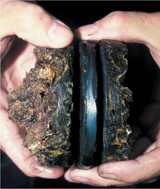
Figure 3. Hull coupon no. USAR-02-001, showing interior and exterior concretion. This sample is from the main deck, outer hull, in water less than 2 m deep with continuous seawater circulation on both sides, which explains thick concretion on both sides and extensive steel corrosion. (Brett Seymour/NPS)
