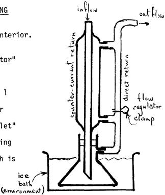
Figure 1: Countercurrent heat exchange simulator.
