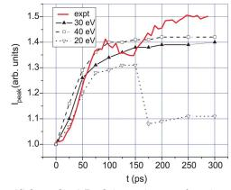
Fig. 3. (Color online) Peak intensity as a function of delay time. The intensity is normalized to the intensity of the undisturbed electron beam. The initial electron density is  $10^{13} \, \mathrm{cm}^{-3}$ . The figure compares experimental data with simulations assuming three different electron temperatures.
