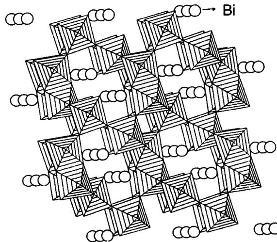
FIG. 2. Projection of the room temperature structure of  $\text{Bi}_2\text{Ti}_4\text{O}_{11}$  deviating  $10^\circ$  from the  $[010]$  direction, the tunnels contain the Bi cations. (This picture was from Ref. 5.)
