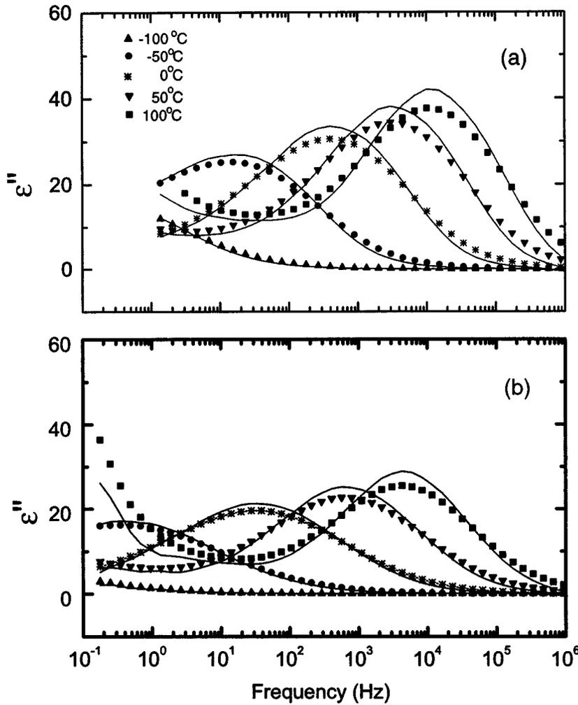
FIG. 6. Comparison of the measured  $\epsilon''$  with the calculated  $\epsilon''$  from Eq. (6) at several different temperatures for BT (a) and BBT (b), where the solid lines represent the calculated results.
