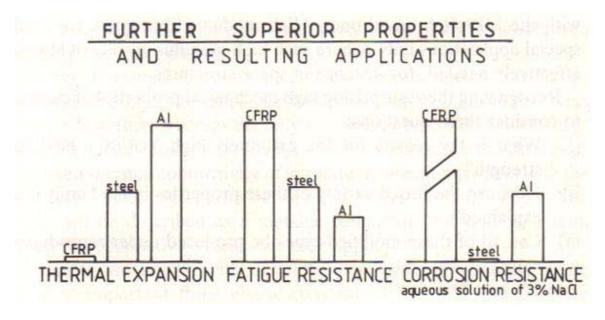
Figure 2. Further advantages properties of advanced composites (CFRP) in contrast to conventional materials.
