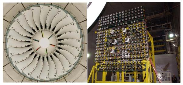
**Engine Inlet Ready for Bird Ingestion Testing**
