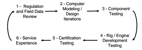
Figure 1 Closed Loop Design Process for Bird Strike Mitigation
