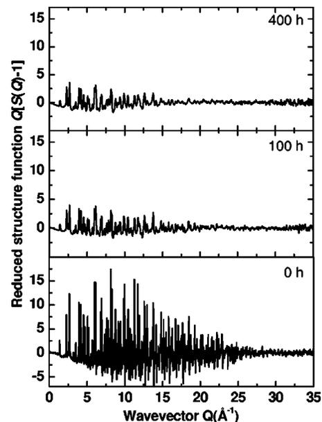
FIG. 3. Reduced structure functions for unmilled  $\text{GdAl}_2$  (bottom) and  $\text{GdAl}_2$  milled for times of 100 h (middle) and 400 h (top).
