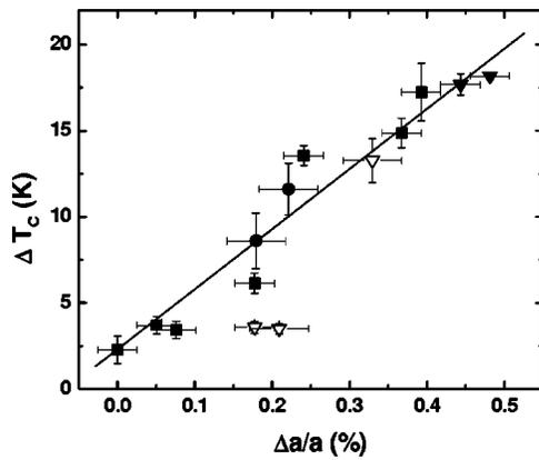
FIG. 9. The dependence of the distribution breadth  $\Delta T_C$  on percent change in lattice parameter in mechanically milled  $GdAl_2$ . Different symbols represent samples from different milling runs. Open symbols represent samples that were milled and subsequently annealed.
