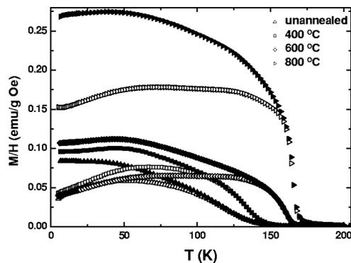
FIG. 12.  $\chi(T)$  for  $GdAl_2$  milled for 590 h (triangles), then annealed 400 °C (squares), 600 °C, (diamonds), and 800 °C (right-pointing triangles). All annealing times were for 10 min with the exception of the 800 °C anneal, which was for 48 h. Open symbols represent ZFC and closed symbols FC measurements.
