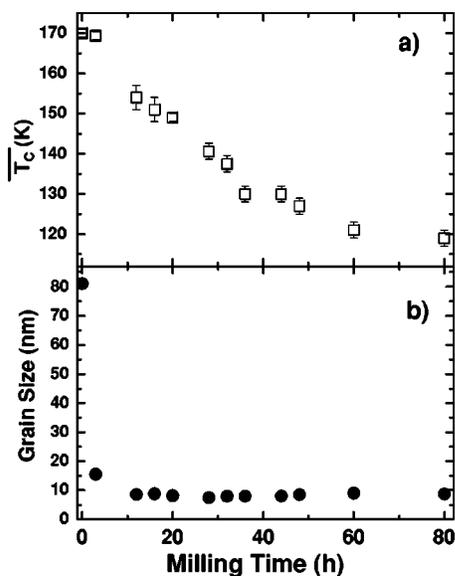
FIG. 7. Changes in (a)  $\bar{T}_C$  and (b) grain size with milling time in mechanically milled GdAl<sub>2</sub>.
