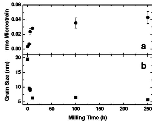
FIG. 2. (a) The root-mean-square microstrain and (b) the grain size as functions of milling time.
