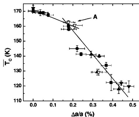
FIG. 8.  $\bar{T}_C$  as a function of percent change of lattice parameter. Different symbols represent samples from different milling runs. The open symbols represent samples milled and subsequently annealed. The letter A refers to a group of points with similar values of  $T_C$  and  $a$ , but very different grain sizes.
