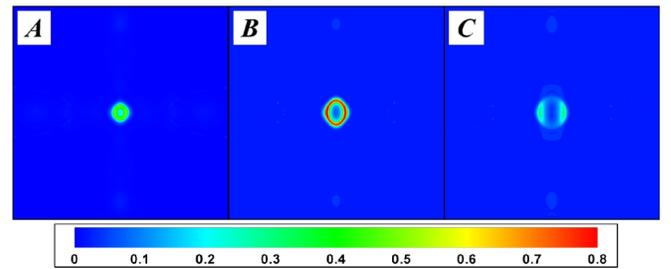
FIG. 3 (color online).  $\mathbf{K}_{\parallel}$ -resolved minority-spin transmission through a Fe/GaAs/Cu (001) tunnel junction for three energies near the maximum at  $E = 106$  meV: (a) 45 meV, (b) 106 meV, (c) 166 meV.
