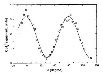
FIG. 7. Parent ion yield as a function of the ellipticity for 800 nm, 80 fs, laser pulses irradiating gaseous toluene, for a fixed peak intensity of 8.5  $\times 10^{13} \, \mathrm{W \, cm^{-2}}$ , measured by varying the angle  $\theta$  between the fast axis of the quarter-wave plate and the polarization direction of incoming linearly polarized light (see text).
