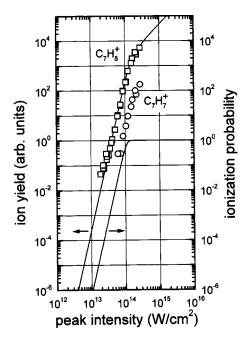
FIG. 2. Ion yields as a function of peak intensity for 800-nm, 80-fs, linearly polarized laser pulses irradiating gaseous toluene. Squares, parent ion,  $C_7H_8^+$ ; circles, fragment ion,  $C_7H_7^+$ . The solid line passing through the parent ion data (left ordinate axis) was obtained by volume-integrating the ionization probability for a six-photon process (lower solid curve, right ordinate axis).
