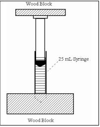
**Now**, an invisible force, namely the weight of the air above the physics lab, is pushing down on the plunger. It is estimated to be about 4.6 kg. If you add 4.6 kg to your values and redraw your graphs. does that make your Cartesian or log-log plot more linear? If it does then find a new equation.
