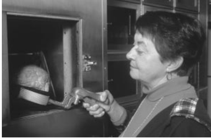
Research Technician Mary Shipman removes a test loaf of bread from the oven at NU's Nebraska Wheat Quality Laboratory. As part of a five-year study, Shipman tested milling and baking qualities of wheat grown using different amounts of fertilizer.
