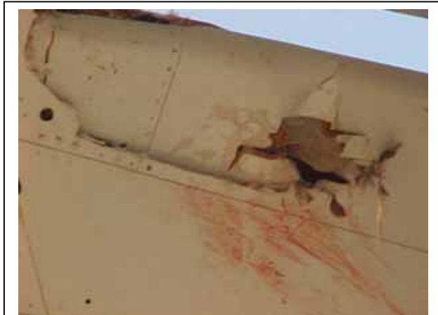
On 30 November 2005 at 1717 hrs and 1200 ft AGL this Boeing 747 struck several birds on approach to a western USA airport, which is located on a major bird migration route. The aircraft sustained damage to the left outboard flap, engines 1 and 2 and a right wing flap fairing. The aircraft was out of service for four days.
