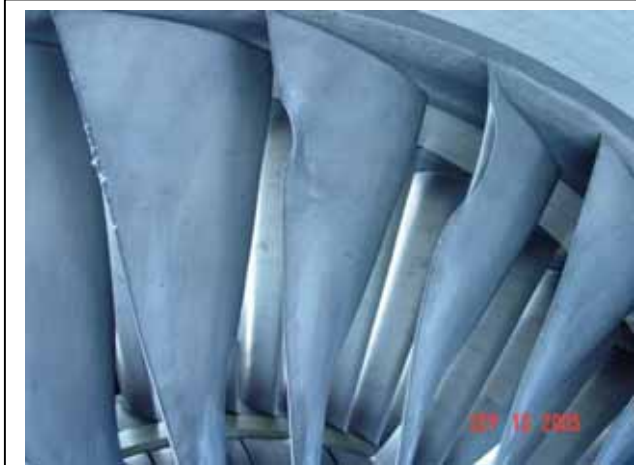
This CRJ600 with 20 passengers on board ingested doves into #1 engine at rotation from a southern USA airport. The engine sustained substantial damage and the aircraft was forced to make a precautionary landing.
