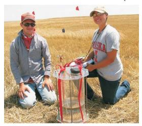
(undergraduate AGEN) assisted Dr. Eisenhauer with research in the Republican River Basin in Kansas. They used this Cornell infiltrometer to simulate rainfall and measure water infiltration.
