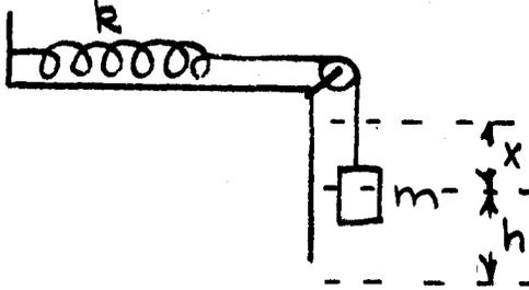
The block in the figure is  $x$  from rest when the spring has its relaxed length. How far does the block descend before coming momentarily to rest.
