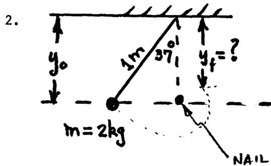
A 2 kg mass is fastened to a 1m string to make a pendulum as shown. The pendulum is released at an angle of  $37^\circ$ . At the center of its swing the string hits a nail and swings on a shorter arc. Using energy conservation, find the distance,  $y_f$ , between the ceiling and the top of the swing on the right hand side.
