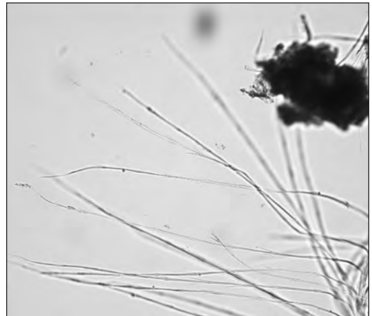
Figure 3. Photomicrograph of a downy feather sample collected from the tail section of the Cessna Citation that crashed near Wiley Post Airport, Oklahoma. The diagnostic microscopic characters of the downy barbs in this sample include short barbules with long, distal prongs.
