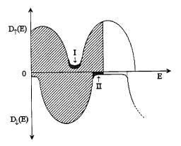
FIG. 1. Schematic ↑ and ↓ densities of states (dark shadowing denotes regions occupied at finite temperature only).
