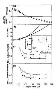
FIG. 4. Evidence of the metamagnetic transition in NiMnSb, taken from (Ref. 54), with permission. (a) Magnetoresistance slope  $[d(\Delta R/R)/d(\mu_0 H)]$ , (b) the resistivity, (c) the relative Ni moment, and (d) relative Mn moment derived from MCD are compared. The change in the magnetic structure factor for the  $\langle 200 \rangle$  peak in neutron scattering shown as an inset, as adapted from (Ref. 55). The  $T^2$  and  $T^{1.65}$  curves are fitted to the resistance data.
