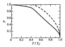
FIG. 2. The temperature dependence of the polarization P, either with (solid) and without (dashed) spin fluctuations for a half metal, adapted from Ref. 43.
