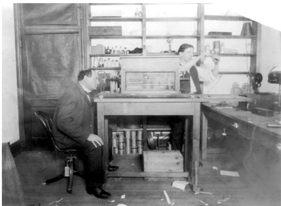
Fig. 2. Dr. Harvey Washington Wiley peering into a saccharimeter in 1902. The box around the device protects it from outside disturbances. (Library of Congress)
