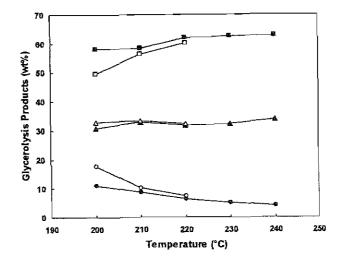
FIG. 1. The effect of reaction temperature and mixing rate on the continuous glycerolysis of soybean oil with pure glycerol, subject to a flow of 40 mL/min and a 2.5:1 molar ratio of glycerol/TG: (**a**), MG; (**a**), DG; and (**9**), TG. Open and solid symbols indicate rotor speeds of 360 and 3600 rpm, respectively.
