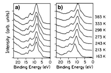
**Fig. 3.** Valence band photoemission spectra taken at normal emission as a function of temperature from a) a  $\sim$ 100 Å thick PVDF film deposited in situ by evaporation and b) nominally 5 monolayer crystalline films of P(VDF–TrFE 70: 30) films fabricated ex situ by Langmuir–Blodgett techniques. The incident photon energy is 42 eV.
