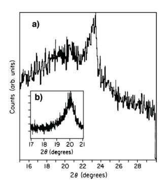
Fig. 2. X-ray diffraction spectra are taken at room temperature using Cu-K $\alpha$  line for a) ~100Å thick PVDF formed by thermal evaporation, and b) a nominally 5 monolayer copolymer P(VDF–TrFE 70:30) film fabricated by the Langmuir–Blodgett technique.
