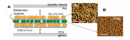
**Fig. 1.** Multilayer structure of electro-optical device. (A) Schematic of the unit structure of the device showing nanoparticle monolayers spaced by an organic DL composed of polyelectrolytes PSS and PAH. A total of three Au and two CdS nanoparticle monolayers with dielectric barriers are deposited. The top Au
