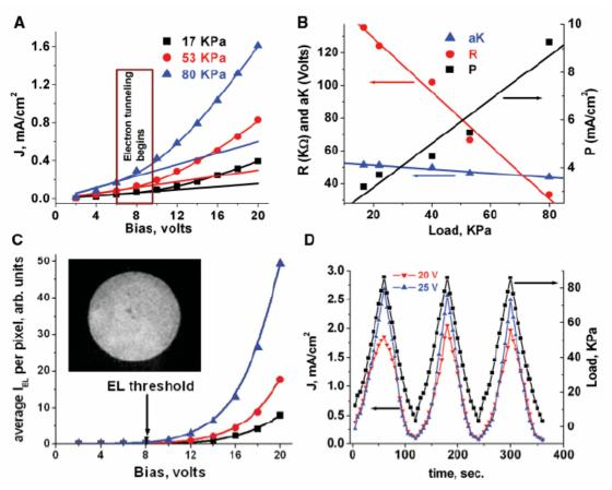
Fig. 2. Electro-optical characteristics of the device and electron-transport mechanism. The device is compressed using an optically flat quartz disk on the flexible Au electrode. (A) J-V data points at various  $\sigma$ . The fitted line is based on
