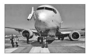
Ryanair Boeing 737-800 in Rome, Italy, after hitting a flock of starlings. Notice bird-strike marks on fuse-lage and the engine (right) resting on the runway.
