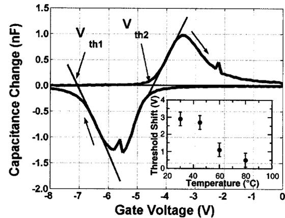
FIG. 2. Derivative of the small-signal capacitance data from Fig. 1 showing the graphical method for determining threshold voltage. Inset: Temperature dependence of threshold voltage shift  $\Delta V_{th} = \Delta V_{th2} - \Delta V_{th1}$ .
