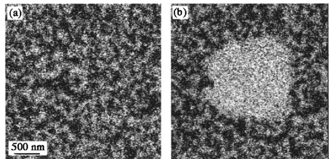
FIG. 3. Piezoresponse images showing the inversion of domains in the thin SBN crystal (a) before and (b) after application of the bias voltage of  $-30$  V.
