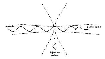
FIG. 1. Schematic of the crossed-laser-plasma wave accelerator concept.
