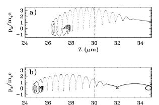
FIG. 13. The same electrons as in Fig. 12; here longitudinal momentum  $p_z/m_e c$  is plotted as a function of position Z. (a) has the electron trapped in the first bucket with (b) showing the particle that bounces before becoming trapped.
