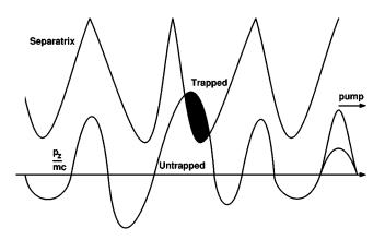
FIG. 3. Basic profile for optical injection. The injection pulse dephases electrons in the plasma wave, distorting it and the separatrix. Electrons cross the separatrix, into the accelerating bucket.
