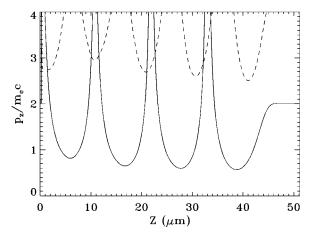
FIG. 15. The minimum trapping threshold, or separatrix. The solid line reflects the minimum momentum needed to trap an electron on axis with the pump pulse. The dashed line is the threshold for the electrons at a radius of  $r_{\rm max}$ =2.5  $\mu$ m from the axis.
