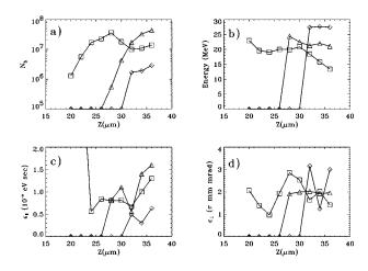
FIG. 16. Beam characteristics as a function of delay between the pump and injection pulses. Shown are (a) number of electrons in the bunch, (b) average energy of the bunch, (c) longitudinal emittance, and (d) transverse emittance. The first bucket is diamonds, second triangles, and third squares.
